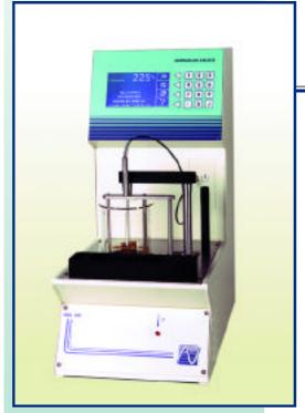
The ultimate Automatic Ring and Ball tester with 2 independant test cells.
