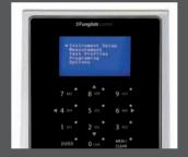
Front view of the viscometer. touch keyboard with 12 keys and graphic display.
